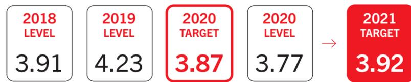
KPI: WATER WITHDRAWN AT THE PLANT (M<sup>3</sup>) / FINISHED PRODUCT (TON)
